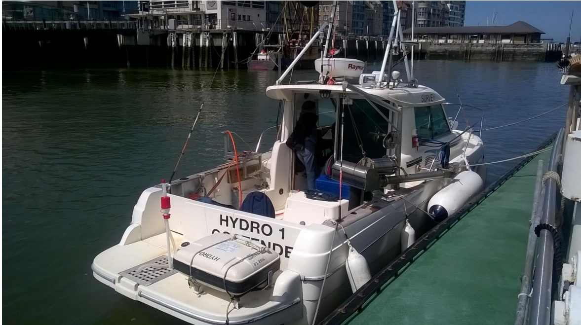
Survey vessel Hydro 1 (Flemish Hydrography). The echosounder pole and orange cable are seen on the left (port side). On starboard side the pole-mounted Octans motion sensor and multibeam unit can be seen.
